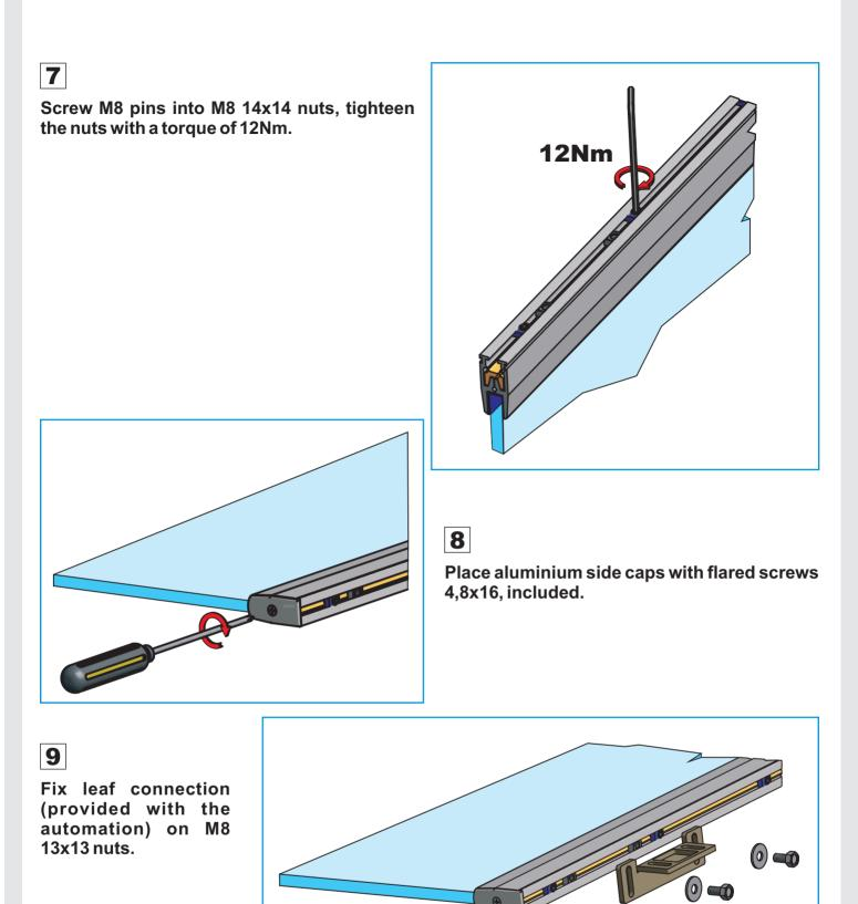
At the end of the installation manually very if the clamps holds properly the glass.
